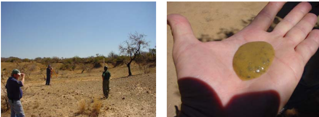
Figure 7. The photo on the left shows an area without topsoil or plant material. The position of the contour is being determined. The photo on the right shows the silicate mineral after water has been added.
