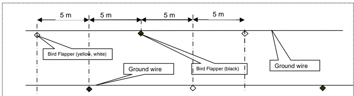
**Figure 7777: Marking method with Bird Flappers on overhead ground wires (viewed from above)**
