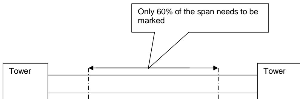
**Figure 8888: The section that needs to be marked**
