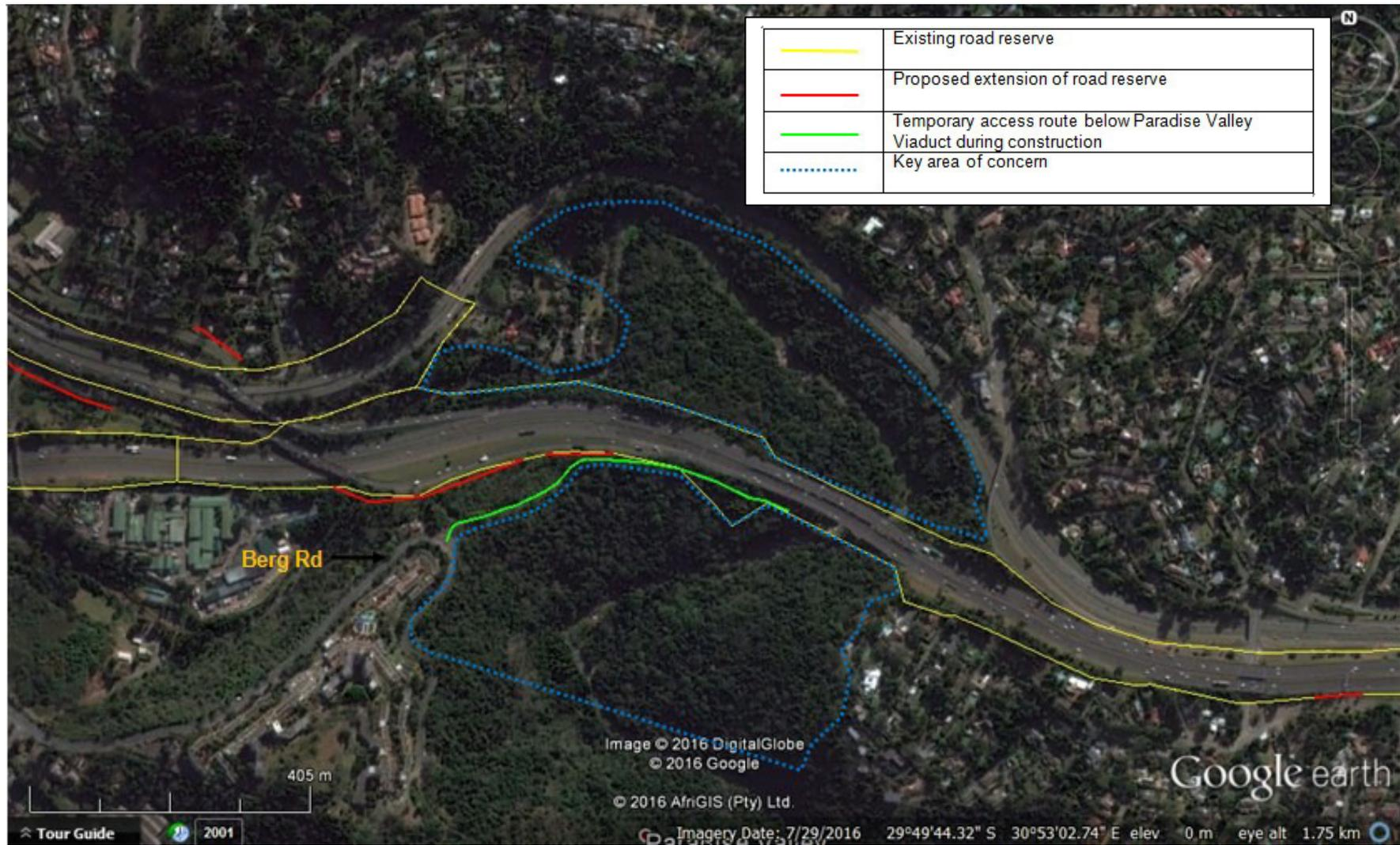
Figure 1 Paradise Valley Viaduct Plan showing temporary access route in green
